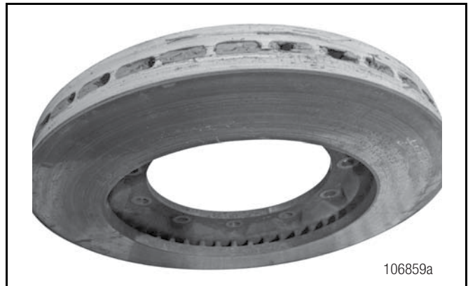
Clogged Vent Holes FIGURE 13
