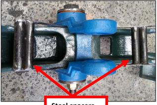
Steel spacers inserted into casting
