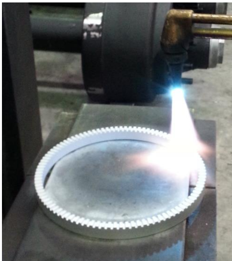
Heating up pole ring using Oxy-Acetylene
