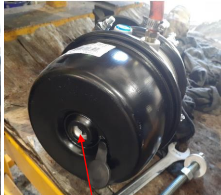
Push rod end visible (ready for cage tool fitment)
