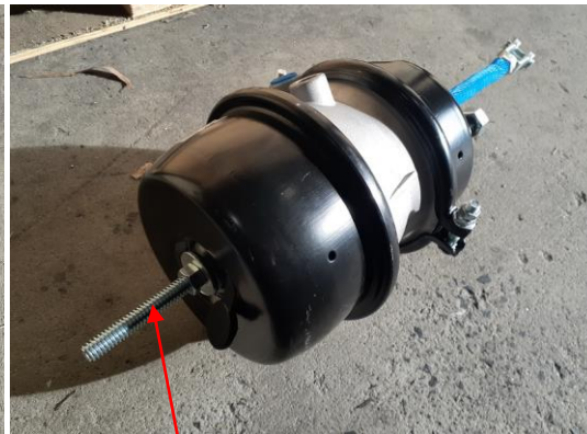
Cage tool fitted to chamber
