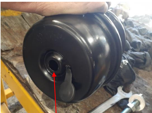
Push rod end not visible (uncaged position)
