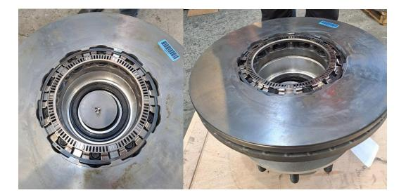
4) Apply a similar procedure in reverse to <u>unassemble</u> the retaining ring from the tabs in the rotor. Use circlip pliers or a flat screwdriver to remove the retaining ring.
