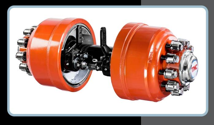
Originally developed in conjunction with Australia's leading specialist low-loader manufacturer for rows-of-eight applications, the UB82 axle for 17.5" wheels can now also be specified with the larger 335mm x 210mm brake (ADR38 rated capacity 11.5 tonne) and at any track length and, in that format, can be fitted to any of TMC's extensive range of airbag or mechanical suspensions.
